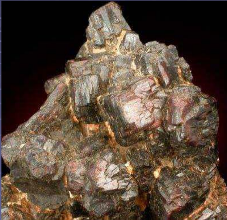
Limonite replacing pyrite (pseudomorph)
